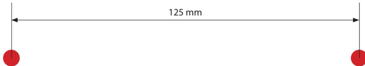
Angaben von Bohrlochmitte zu Bohrlochmitte // Measurements from centre of one drill hole to the other //
